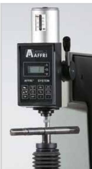
Hardness testing machine. Metal and rubber materials.
