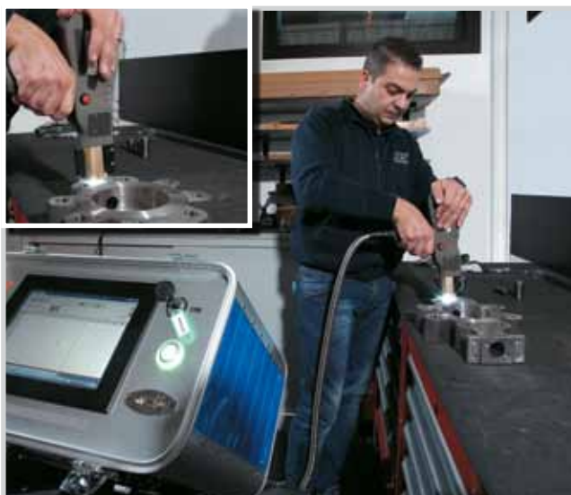
Optical emission spectrometer. PMI testing (Positive Material Identification)
