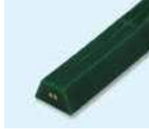
Result after overlap welding
