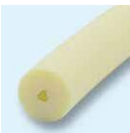
63° Shore D · approx. >100° Shore A Recommended pretension 0,5...2 %
