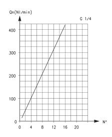
Flow Qn (Nl/min.) from 2  $\rightarrow$  1 with controller OPEN: 200 Flow Qn (Nl/min.) from 2  $\rightarrow$  1 with controller CLOSED: 70
