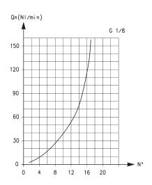
Flow Qn (Nl/min.) from 2  $\rightarrow$  1 with controller OPEN: 70 Flow Qn (Nl/min.) from 2  $\rightarrow$  1 with controller CLOSED: 33
