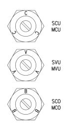
**IDENTIFICATION OF DIFFERENT TYPES:** SCU - MCU = assembly directly on the cylinders SVU - MVU = assembly directly on the valves SCO - MCO = assembly directly on the cylinders or valves
