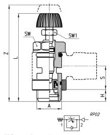
Note: M5 flow controllers must be used together with M6 adjustable fittings.
