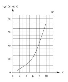
Flow Qn (NI/min.) from  $2 \rightarrow 1$  with controller OPEN: 70 Flow Qn (Nl/min.) from 2 → 1 with controller CLOSED: 33 Qn = supply pressure of 6 bar and with  $\Delta P$  = 1 bar at the outlet N° = number of screw turns.
