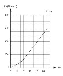
Flow Qn (NI/min.) from  $2 \rightarrow 1$  with controller OPEN: 440 Flow Qn (NI/min.) from  $2 \rightarrow 1$  with controller CLOSED: 170
