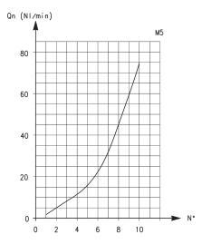
To ensure the right choice of unidirectional flow controller, proceed as follows: calculate the quantity of air in NI/min (see cylinder Table); determine the stroke time of the cylinder; refer to graph to see which controller is the right type.
