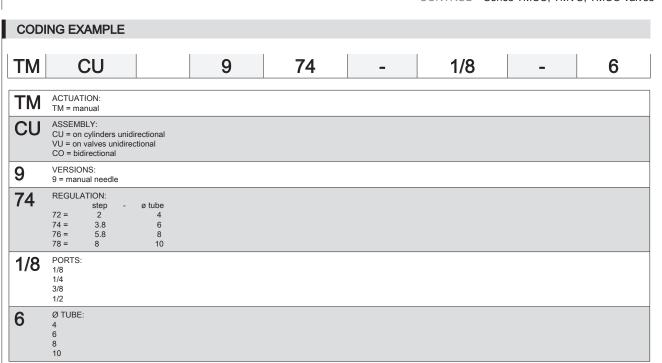
To ensure the right choice of unidirectional flow controller, proceed as follows: calculate the quantity of air in NI/min (see cylinder Table); determine the stroke time of the cylinder; refer to graph to see which controller is the right type.
